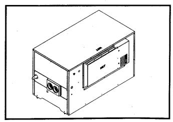
FIG. 11 Outdoor Vent Cap Installed on Unit
