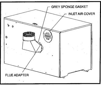
FIG. 14 Installation of Flue Adapter and Inlet Air Cover
