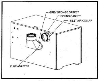
FIG. 13 Installation of Flue Adapter and Air Inlet Collar
