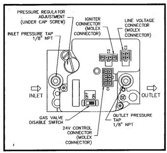
FIG. 45 SmartValve Combination Gas Valve
