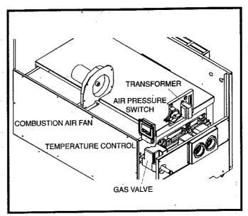
FIG. 42 Component Location Drawing
