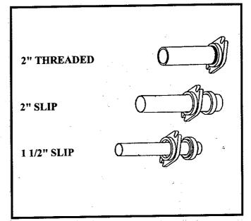
FIG. 39 Alternate Piping Connections
