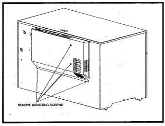
FIG. 12 Removal of Outdoor Vent Cap
