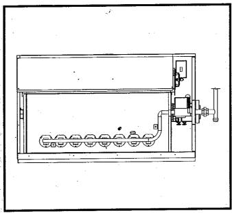
FIG. 49 Gas Train and Burners
