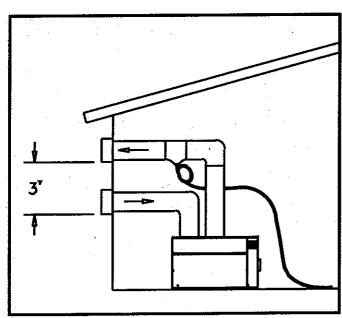
FIG. 28 E-Rite Sidewall Vent Installation
