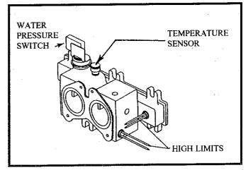
FIG. 44 Front Header with Limits, Pressure Switch and Temperature Sensor
