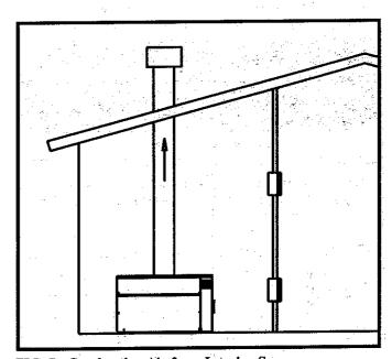
FIG. 7 Combustion Air from Interior Space
