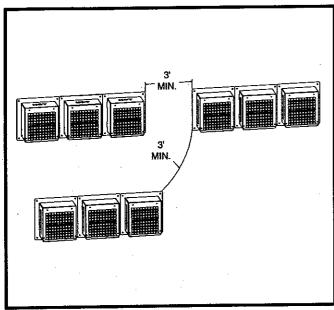
FIG. 32 Installation of Multiple E-Rite Sidewall Vent Caps
