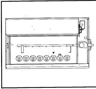
FIG. 50 · Gas Train Rotated Up for Burner Removal
