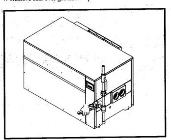
FIG. 34 Wrench to Support Gas Valve for Piping Connection
