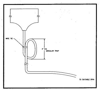
FIG. 31 Drain Tee Installation
