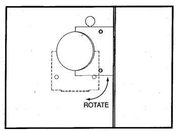
FIG. 53 Access and Positioning of Wiring Grommet
