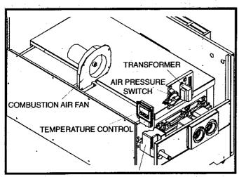
FIG. 54 Combustion Air Fan Location
