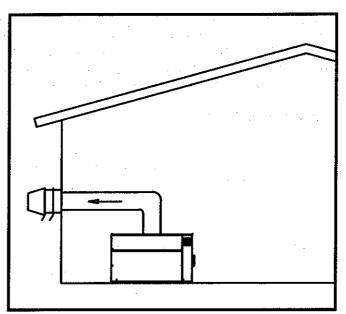
FIG. 24 Sidewall Venting Installation with Powered Vent Cap
