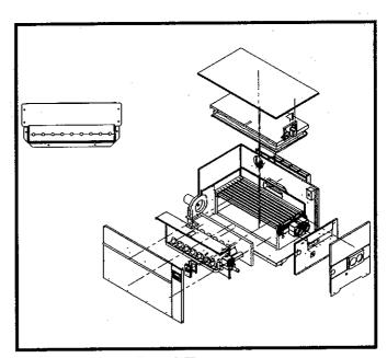
FIG. 51 Exploded View of Heater
