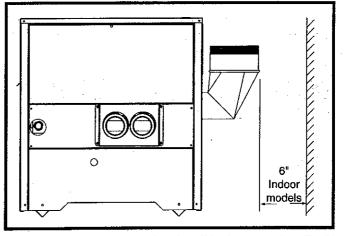
FIG. 4a Clearances from Combustible Construction (Back) Clearances from Combustible Construction:
