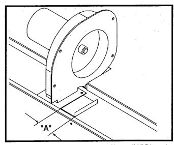
FIG. 29 Combustion Air Fan with Air Shutter "A" Dimension
