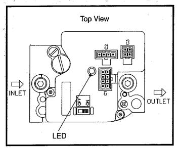
FIG. 47 Top View of SmartValve and LED Indicator
