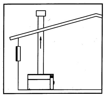
FIG. 8 Combustion Air from Outside - Single Opening
