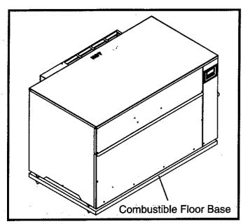
FIG. 3 Special Combustible Floor Base
