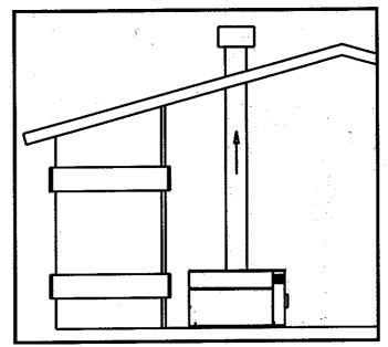
FIG. 6 Combustion Air Through Ducts
