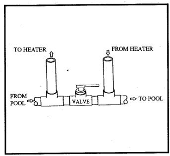
FIG. 40 Auxiliary Bypass Piping
