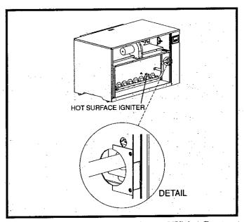
FIG. 52 Access to Hot Surface Igniter and Wiring Grommet
