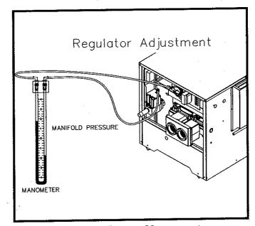
FIG. 36 Manifold Gas Pressure Measurement
