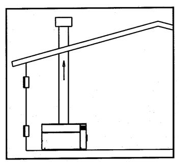
FIG. 5 Combustion Air Direct from Outside
