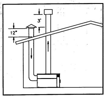
FIG. 22 Vertical DirectAire Installation with Roof Top Combustion Air
