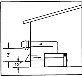
FIG. 26 Power Horizontal DirectAire Installation Illustration
