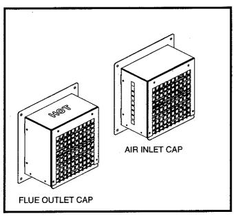
FIG. 30 E-Rite Sidewall Vent Caps Illustration
