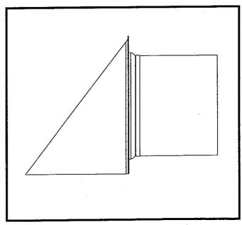
FIG. 27 Air Inlet Cap for Sidewall Termination
