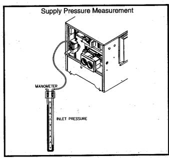
FIG. 37 Gas Supply Pressure Measurement at Combination Gas Valve
