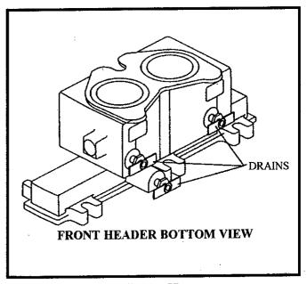
FIG. 60 Front Header - Bottom View
