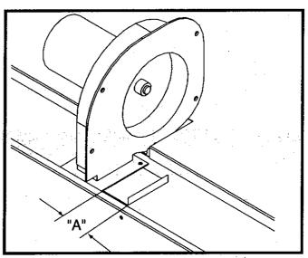
FIG. 55 Combustion Air Fan with Air Shutter "A" Dimension
