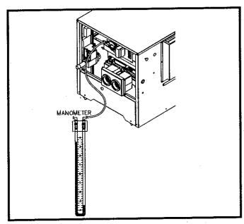
FIG. 35 Front Chamber Pressure Measurement
