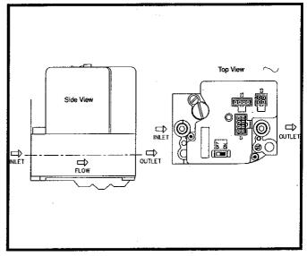
FIG. 46 SmartValve with Hot Surface Ignition Control Module
