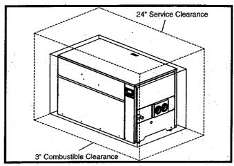
FIG. 4 Clearances from Combustible Construction (Front)
